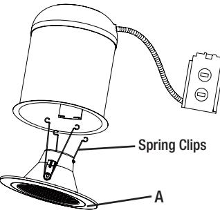
**7** Connect the connector cable from the medium base (E26) socket adapter to the connector cable from the fixture.
