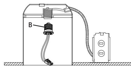
**6** Screw the medium base (E26) socket adapter into the socket in the can.
