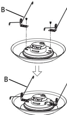
**4a** Installing into a recessed can: Attach the spring clips to the fixture.
