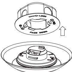
**6b** Secure the fixture to the mounting plate by inserting the fixture into the keyholes on the mounting plate and twisting the fixture until it is secure.
