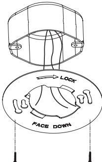
**4b** For surface mounting: Attach the mounting plate to the J-Box.
