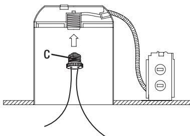
**5a** Screw the medium base (E26) socket adapter into the socket in the can.
